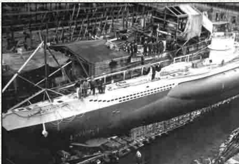
Above (3): The division between the lighter upper grey and the lower darker grey can clearly be seen on U 69. As was common practice, the whole of U 69's saddle tanks were painted in the lower anti-fouling colour.
