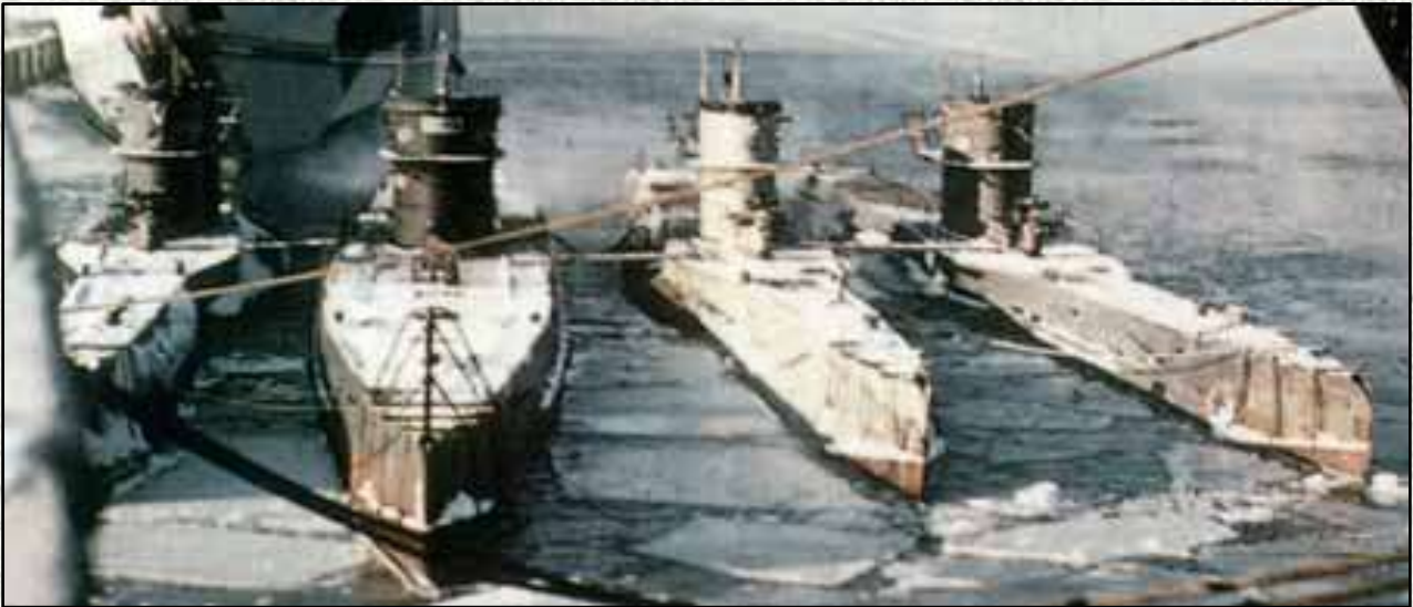
Above (7): The U-boats seen here in Gotenhafen have rusty protective caps over their bows to prevent damage from ice. The decks are covered under a layer of snow. The Type IX second from the left, U 37, looks particularly
