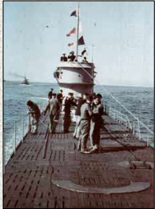
Above (18): The pristine looking Type IX U 128, with a Hellgrau 50 tower, in May 1941. The freshly-stained wooden deck looks dark, with only a tinge of brown showing through. The metal hatch on the right of the photo, and the C-shaped metal part at the bottom of the photo, have been painted black.
