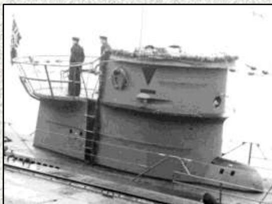
Above (E6): The standard magnetic compass fairing on U 408. As the photo illustrates, the fairing abutted the front of the tower.
