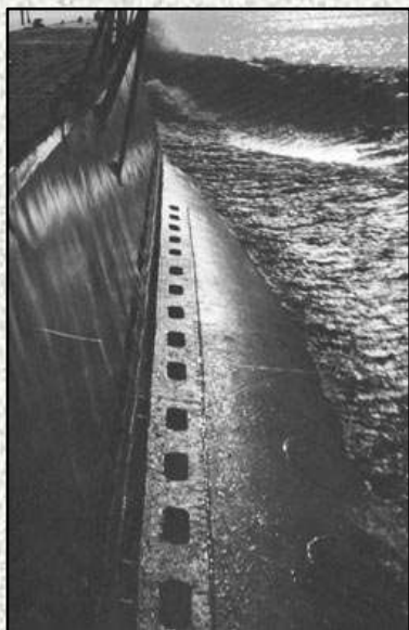
Above left (D44): Another exclusive feature of the IIDs is the line of vents at the very top of the saddle tanks. In this photo we can see the position of the vents just outboard of the main drainage area. Below (D45): The arrows show the position of the various vents on top of the saddle tanks. U 141 had an additional seven vents towards the rear end of the tank. These extra vents were a little smaller than the other 26 vents.
